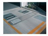
BM7010 is a strong in-ground brake tester for light vehicles with axle loads up to 3500 kg. The design of the BM7010 is unique on the market due to the "split roller bed" system. The brake tester roller set is hot-galvanized and together with the aluminium display, it can be installed both in- and outdoors.
